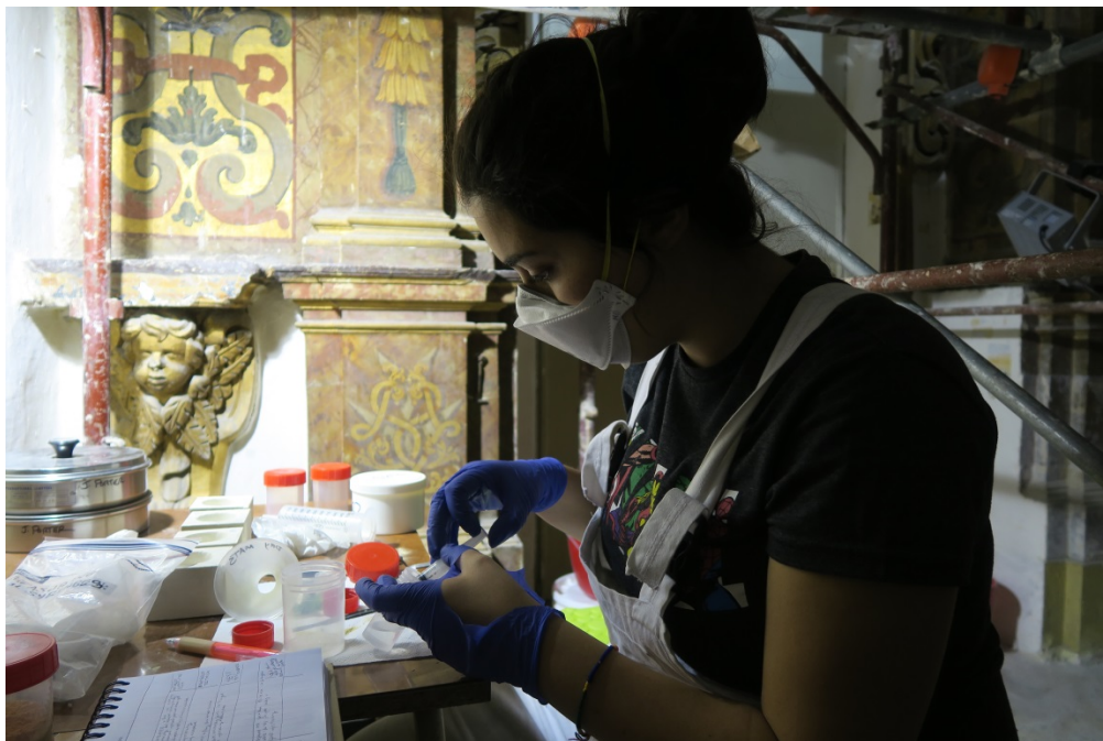
Nathalie Debono developing a material for the stabilisation of detached plaster (©DCBH, UM)
